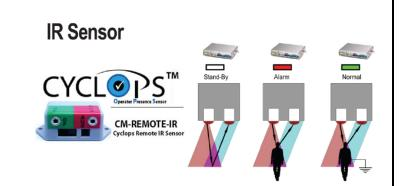
**CYCLOPS<sup>™</sup> Infrared Operator Presence Sensor** CYCLOPS<sup>™</sup> assure compliance with personnel grounding requirements and protect ESD safe workstations by sensing when an operator is within the protected work area. An operator who approaches the workstation without connecting their wrist strap causes the monitor to alarm. The alarm continues until compliance is achieved, preventing isolated operators from damaging ESD sensitive devices.
